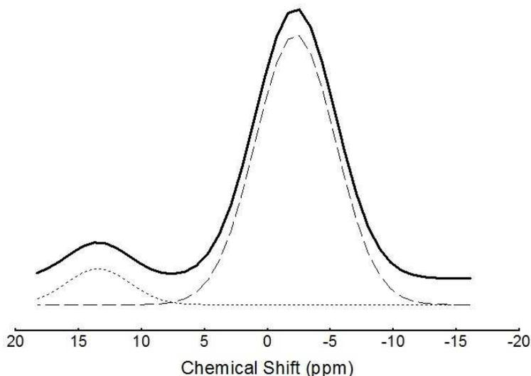
**Figure 6.** Deconvolution of NMR spectra for glass of 20 mol % CdO. solid lines denote experimental  $^{51}\text{V}$  MAS NMR data, and filled curves or dashed lines represent fitting of the data using Gaussian line shape.
