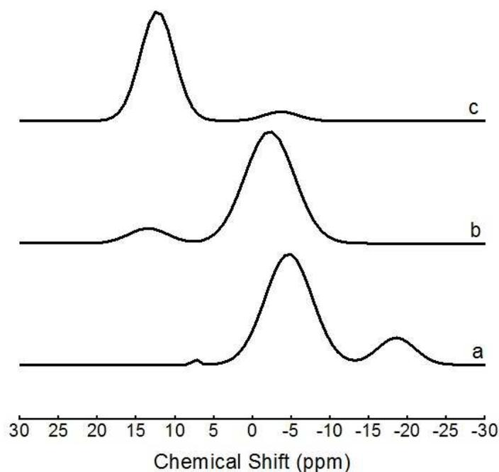
**Figure 5.**  $^{31}\text{P}$  MAS NMR spectra for ternary CdO- $\text{V}_2\text{O}_5$ - $\text{P}_2\text{O}_5$  glasses containing 0, 20 and 30 mol% CdO represented by spectra (a), (b), and (c) respectively.
