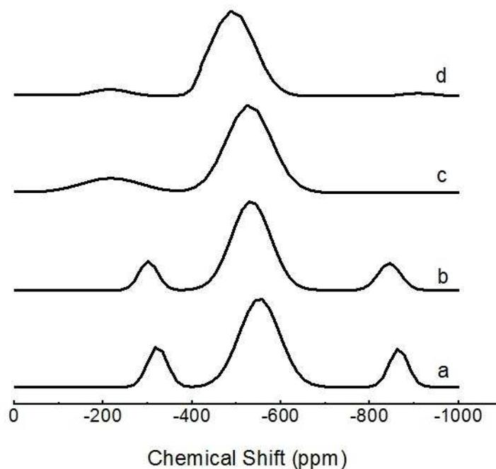
**Figure 3.**  $^{51}\text{V}$  MAS NMR spectra for ternary  $\text{CdO-V}_2\text{O}_5\text{-P}_2\text{O}_5$  glasses containing 0, 20, 30 and 50 mol% CdO represented by spectrum (a), (b), (c), and (d), respectively.
