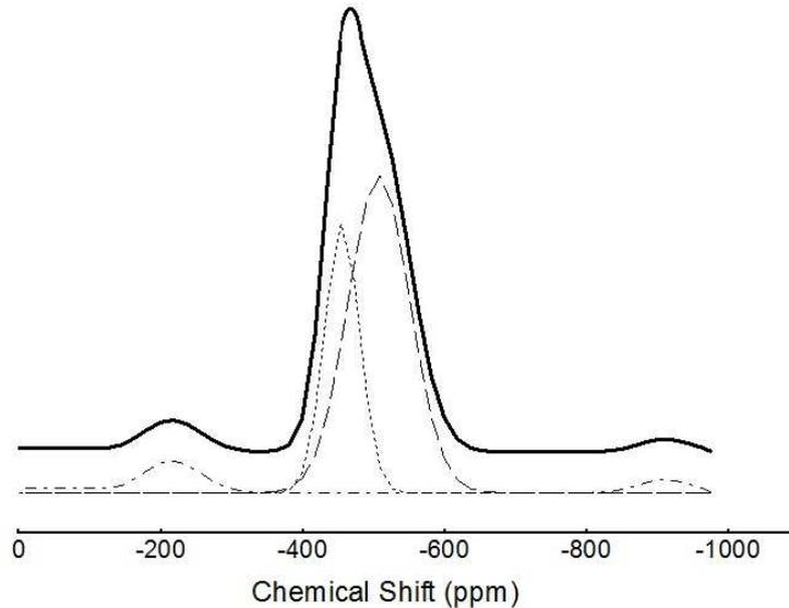
**Figure 4.**  $^{51}\text{V}$  MAS NMR deconvoluted spectra for glass containing 50 mol% CdO as an example.
