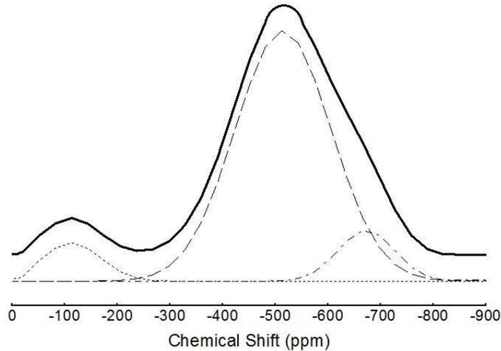
**Figure 2.** Deconvolution of NMR spectra for glass of 60 mol% CdO, solid lines denote experimental  $^{51}\text{V}$  MAS NMR data, and filled curves or dashed lines represent fitting of the data using Gaussian line shapes.
