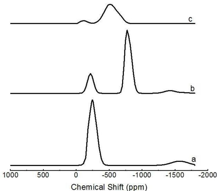
**Figure 1.**  $^{51}\text{V}$  MAS NMR spectra for CdO- $\text{V}_2\text{O}_5$  glasses with composition (a) the vitreous ( $\text{V}_2\text{O}_5$ ), (b) and (c) for the binary CdO- $\text{V}_2\text{O}_5$  glasses containing 30 and 60 mol% CdO, respectively.
