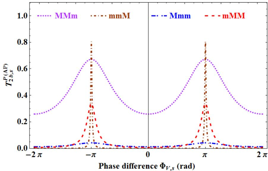
**Figure 5.** The transmission coefficients as a function of the phase difference  $\Phi_{V,s}$  under applied voltage of  $V = 0.01$  V are shown. The curves are calculated with the same parameters as in Fig. 3. The four curves correspond to the spin conduction channels of electron.
