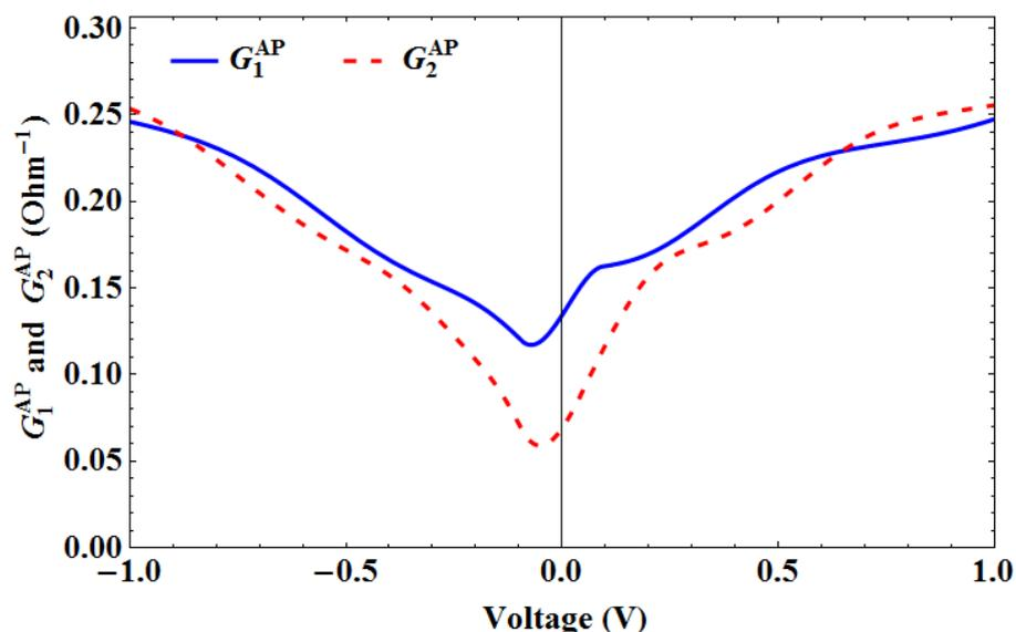
**Figure 7.** Dependencies of the tunnel conductances vs applied bias out of plane in the asymmetrical DAMTJ for two MmM+mmM (solid line) and Mmm+mMM (dashed line) of different channels at room temperature.
