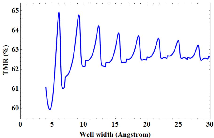
**Figure 8.** The tunnel magnetoresistance as a function of the middle ferromagnetic layer  $\text{FM}^w$  thickness  $L_w$  in the case of  $V = 0.01 \text{ V}$ , calculated with the same parameters as in Fig. 3.
