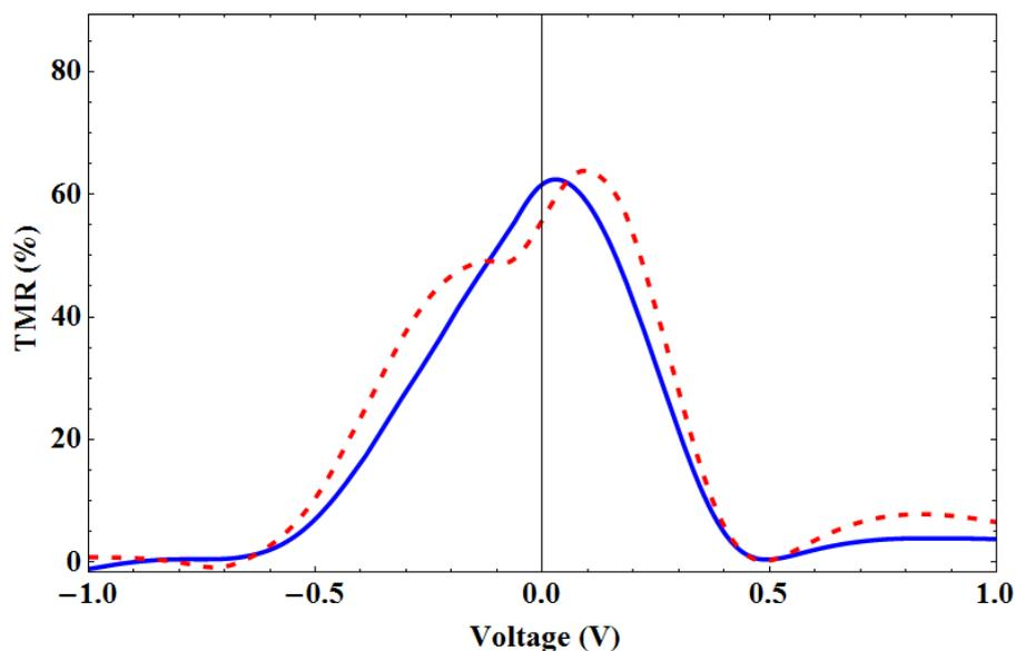
**Figure 9.** Bias dependence of TMR for  $L_w=25.0 \text{ \AA}$ . The dashed curve is obtained at the maximum value of the transmission coefficient, see formula (10). The other parameters at which the obtained TMR curves are the same as in Fig. 3.
