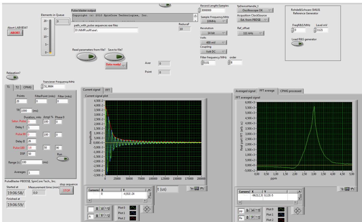
Figure 4. Program interface and  $^1\text{H}$  NMR signal (left) and spectrum (right).
