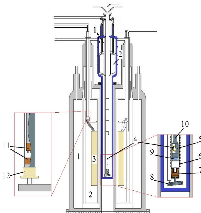
**Figure 2.** The magnet and the cryostat. Nitrogen vessel (1); helium vessel (2); superconducting magnet (3); NMR-coil with sample (4); thermostating chamber (5); shield (6); heat exchanger (7); stainless steel capillary (8); heating element (9); stainless steel support (10); 18-pin connector to magnet system (11); 32-pin connector to magnet system (12).
