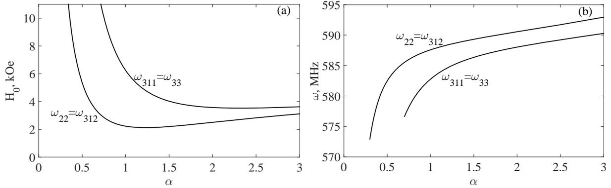
**Figure 3.** Dependence of magnetic field (a) and degenerated frequencies (b) on the shape parameter of the sample
