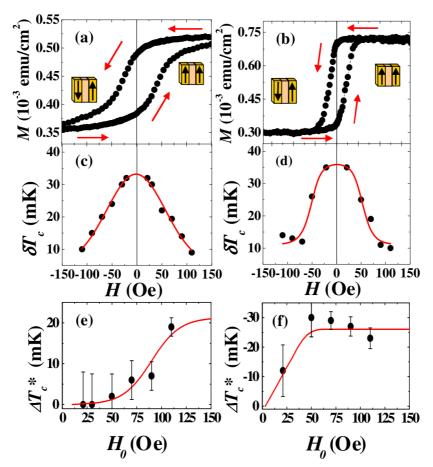
Figure 4. (Color online) The minor hysteresis loops for the spin valve samples with  $d_{\text{Fe2}} = 0.5 \text{ nm}$  (a) and  $d_{\text{Fe2}} = 1.3 \text{ nm}$  (b) and the dependencies of  $\delta T_c$  and  $\Delta T_c^*$  on the magnetic field value: the panels (c) and (e) correspond to the sample with  $d_{\text{Fe2}} = 0.5 \text{ nm}$  and the panels (d) and (f) correspond to the sample with  $d_{\text{Fe2}} = 1.3 \text{ nm}$  [32, 33].
