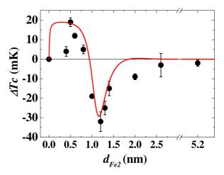
**Figure 5.** (Color online) The dependence of the  $T_c$  shift  $\Delta T_c = T_c^{AP} - T_c^{P}$  on the Fe2-layer thickness  $d_{\text{Fe2}}$ . The applied switching field  $H = \pm 110$  Oe. Theoretical curve (solid line) corresponds to the calculated function [W(0)-W( $\pi$ )]/W(0) (see [38]) normalized to our experimental data [32, 33]
