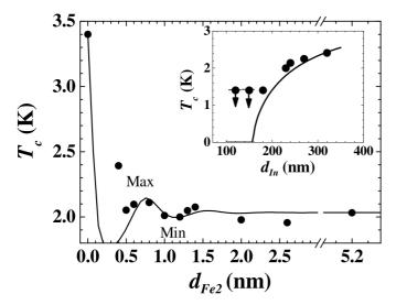
Figure 6. Superconducting transition temperature  $T_c$  versus the Fe2-layer thickness  $d_{\rm Fe2}$  for the spin valve system  $\rm CoO_x/Fe1/Cu/Fe2/In$  with a fixed thickness of the In layer  $d_{\rm In} = 230$  nm. Inset shows the dependence of  $T_c$  on  $d_{\rm In}$  for the set of the samples with a fixed thickness of the Fe layer  $d_{\rm Fe2} = 3$  nm. Solid lines are theoretical fits (see the text) [33].
