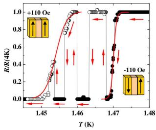
Figure 3. (Color online) Switching between normal and superconducting states in the spin valve sample #3 during a slow temperature sweep by applying the magnetic field  $H_0 = -110 \text{ Oe}$  (closed circles) and  $H_0 = +110 \text{ Oe}$  (opened circles) in the sample plane [32,33].
