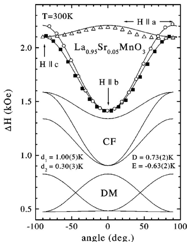
**Figure 4.** Angular dependence of the EPR linewidth in  $\text{La}_{0.95}\text{Sr}_{0.05}\text{MnO}_3$  for the magnetic field applied within the three crystallographic planes at 300 K. The solid lines represent the fit. The lines below illustrate the contributions of crystal field (CF) and Dzyaloshinsky-Moriya (DM) interaction, respectively.
