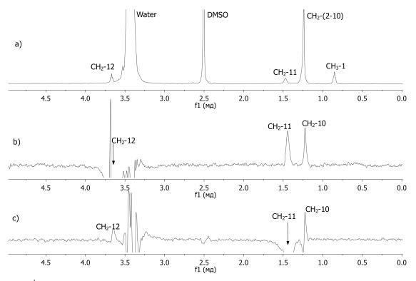
**Figure 2.** <sup>1</sup>H NMR (500.13 MHz) spectrum (a) and selective 1D NOESY spectra (b, c) of SDS in DMSO+H<sub>2</sub>O solution at T = 298 K (concentration 2 g/l). The arrow shows the signal with the frequency of applied selective RF pulse. Mixing time is  $\tau_{\rm M} = 400$  ms.
