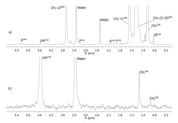
**Figure 5.** Selective 1D NOESY spectrum (b) and <sup>1</sup>H NMR (500.13 MHz) spectrum (a) of cholesterol+SDS mixture in DMSO+H<sub>2</sub>O solution at T = 298 K. Mixing time is  $\tau_{M} = 50$  ms. The chemical structures of cholesterol and SDS molecules with atom numeration are also shown on the figure. The arrow shows the atoms for which Overhauser effect is observed.
