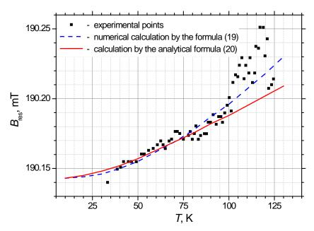
**Figure 2.** Temperature dependence of the resonance field (for  $H \perp c$ ) in YBCO<sub>6.1</sub> with 2% of Yb: experimental points are marked by squares, dashed line gives the numerical calculation by the formula (19) for  $g_{Yb}^0 = g_{\perp}^0 = 3.4$  and solid line is the calculation by the analytical formula (20).
