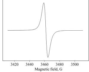
Figure 1. EPR spectrum measured at room temperature for the polymeric complex of the VT-AN copolymer with AgNO<sub>3</sub>, where  $g_{\parallel} = 2.2623(2)$ ,  $g_{\perp} = 2.0762(2)$ .
