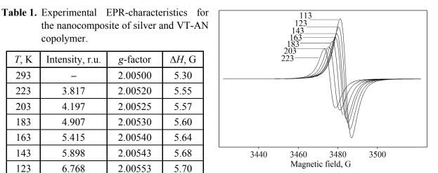
Figure 5. Temperature dependency (K) EPR spectra of the nanocomposite of silver and VT-AN copolymer.
